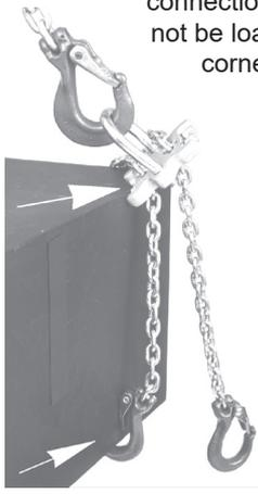
Load hooks must not be loaded on the tip.
