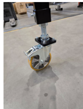
Vertically adjustable leg and wheel in movable workstations crane
