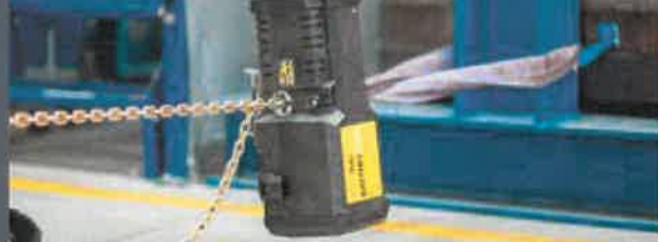
Horizontal pulling by remote control, also in places without power supply.
